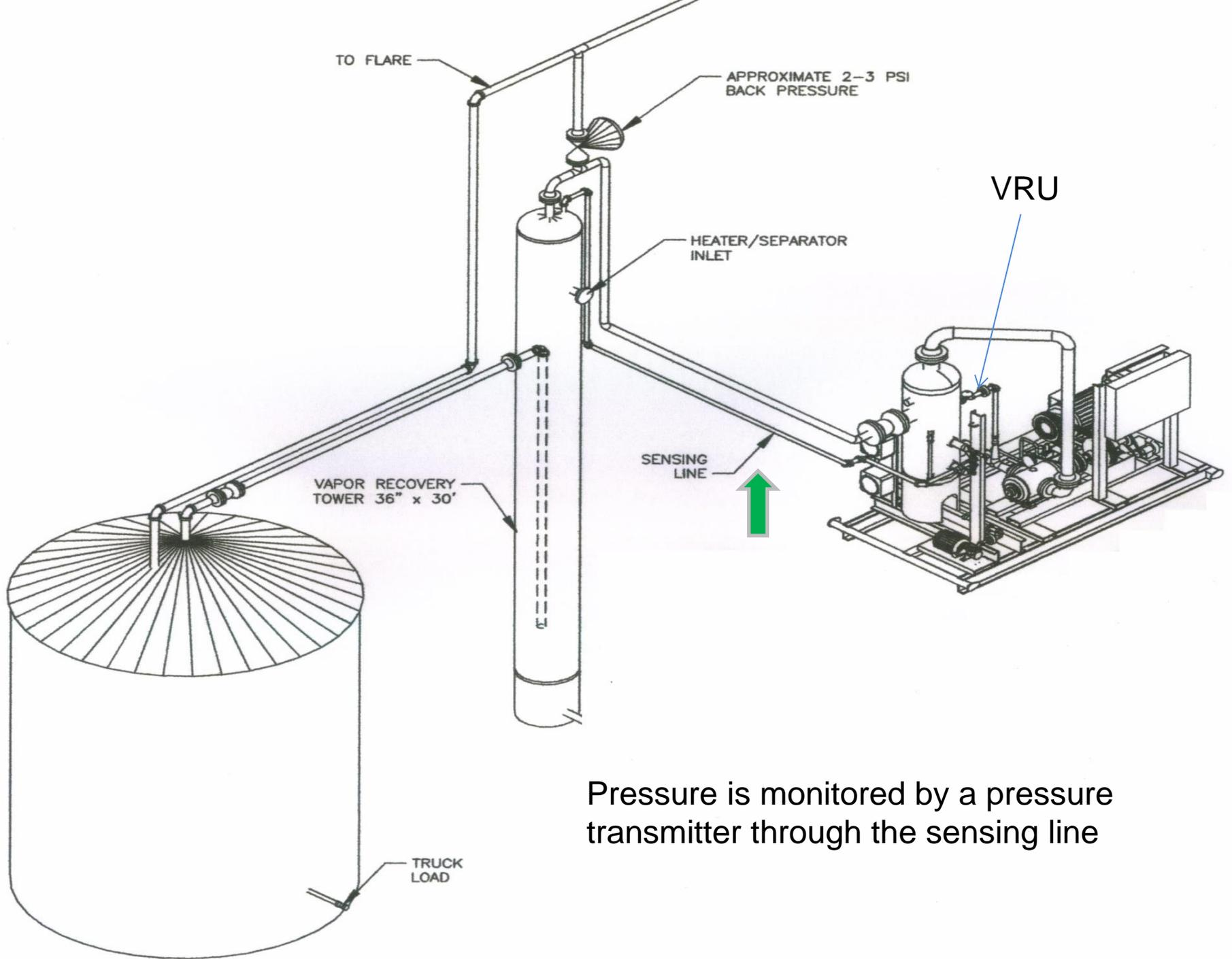
Pressure is monitored by a pressure transmitter through the sensing line
