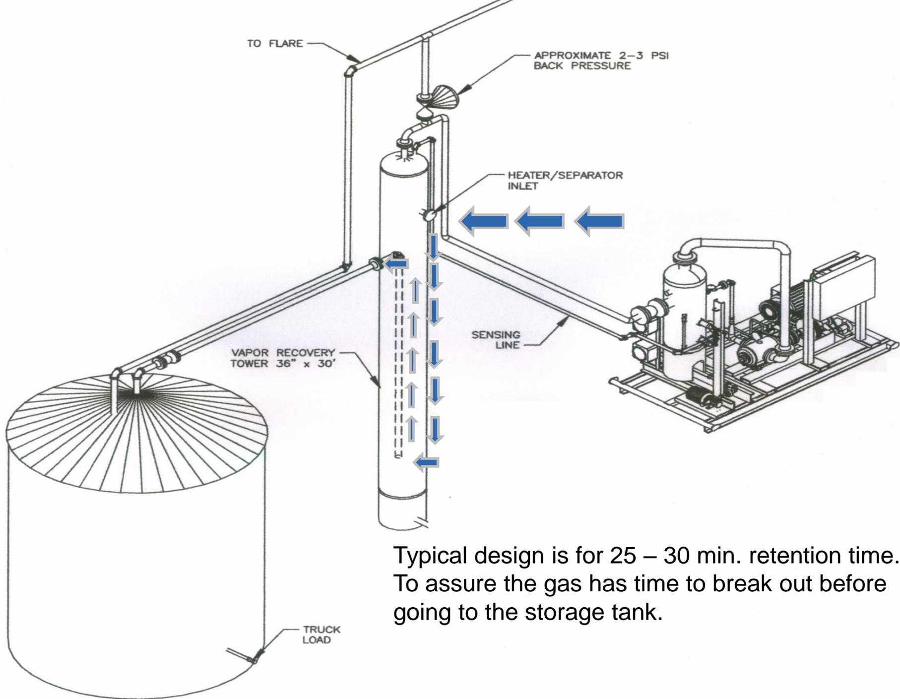
Typical design is for 25 – 30 min. retention time. To assure the gas has time to break out before going to the storage tank.
