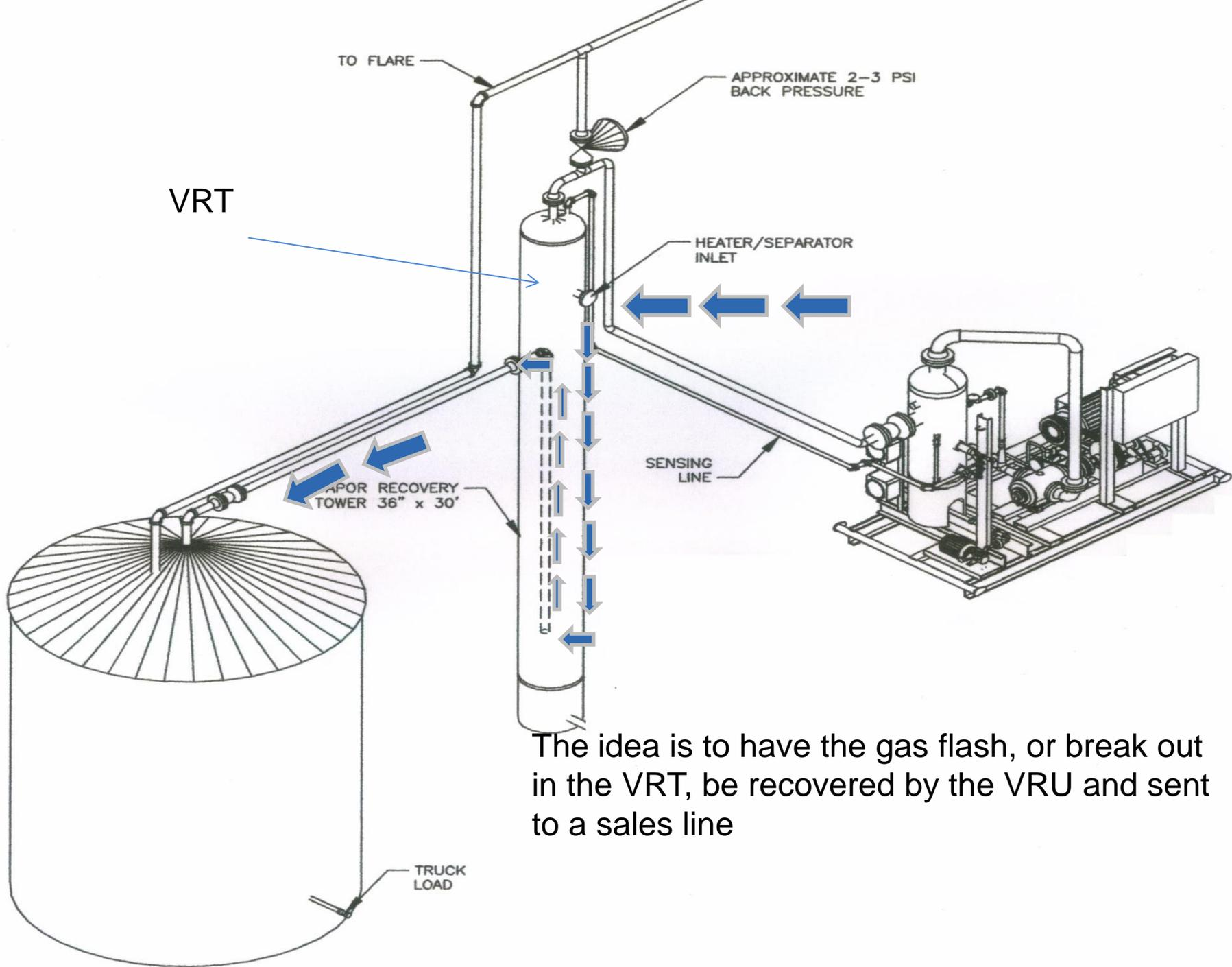
The idea is to have the gas flash, or break out in the VRT, be recovered by the VRU and sent to a sales line
