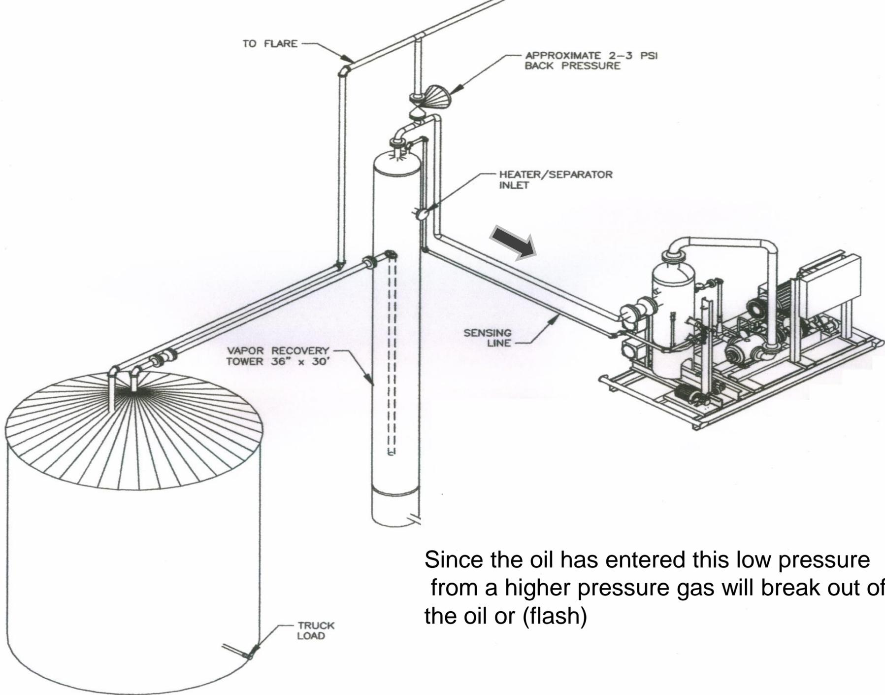
Since the oil has entered this low pressure from a higher pressure gas will break out of the oil or (flash)
