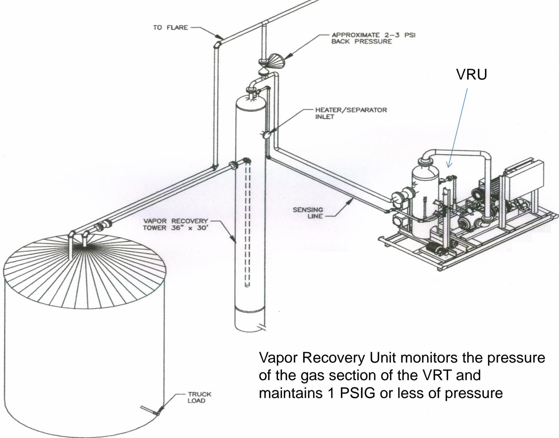
Vapor Recovery Unit monitors the pressure of the gas section of the VRT and maintains 1 PSIG or less of pressure
