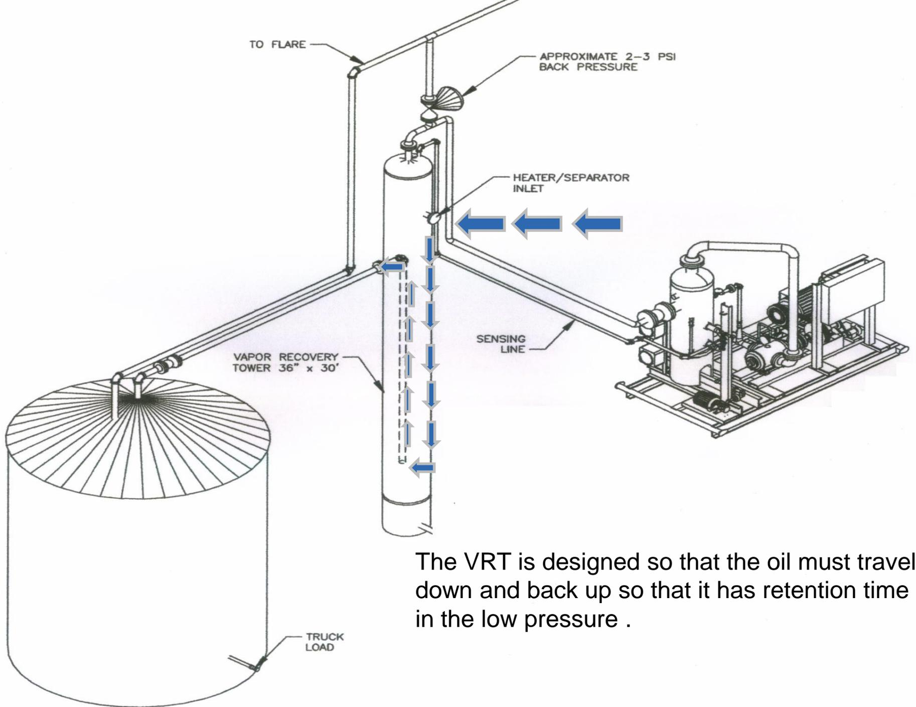
The VRT is designed so that the oil must travel down and back up so that it has retention time in the low pressure .
